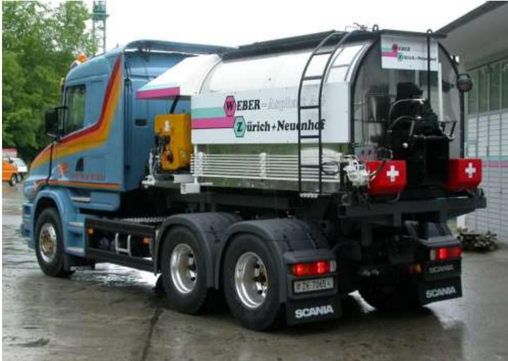
*Figure 6: Mastic asphalt mixer for transportation with horizontal mixing system.*
