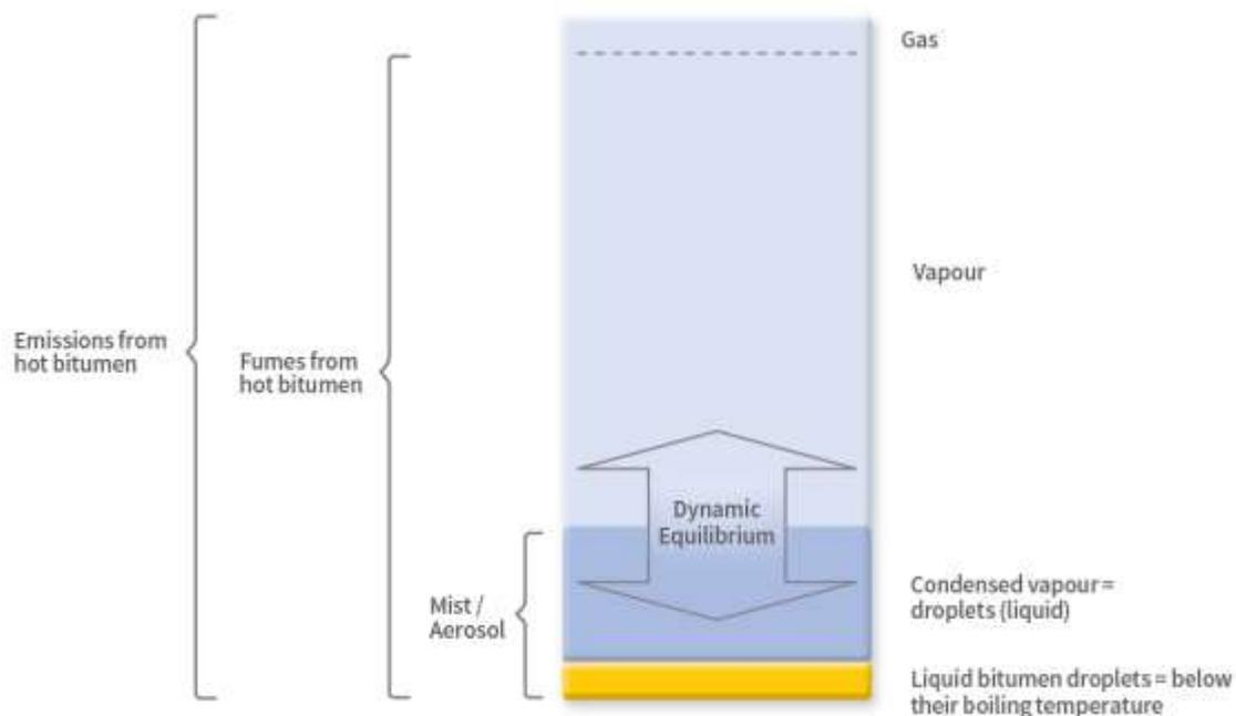
Figure 9: Schematic diagram of bitumen emissions composition [3].
