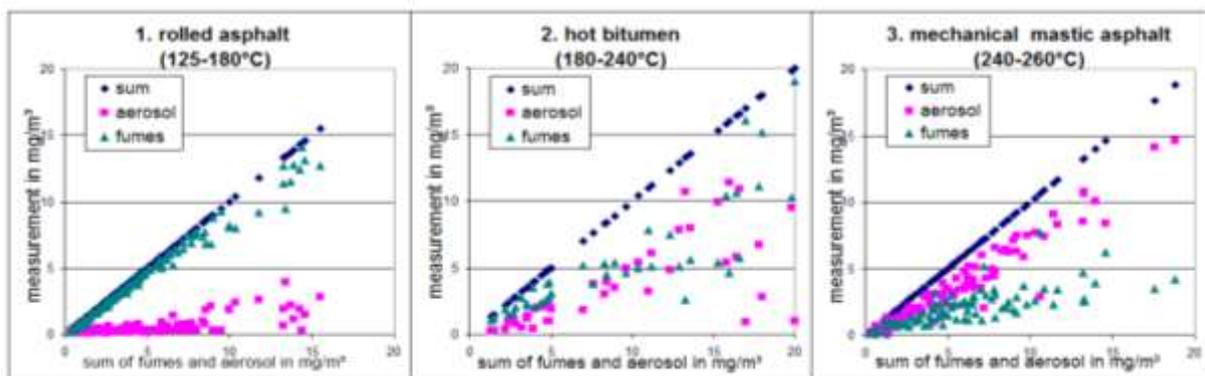
Figure 16: Distribution of bitumen vapours and aerosols according to application temperature [13]
