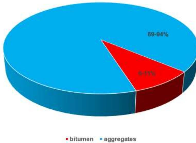
Figure 5: Mastic Asphalt Current Components (Schematic Diagram)
